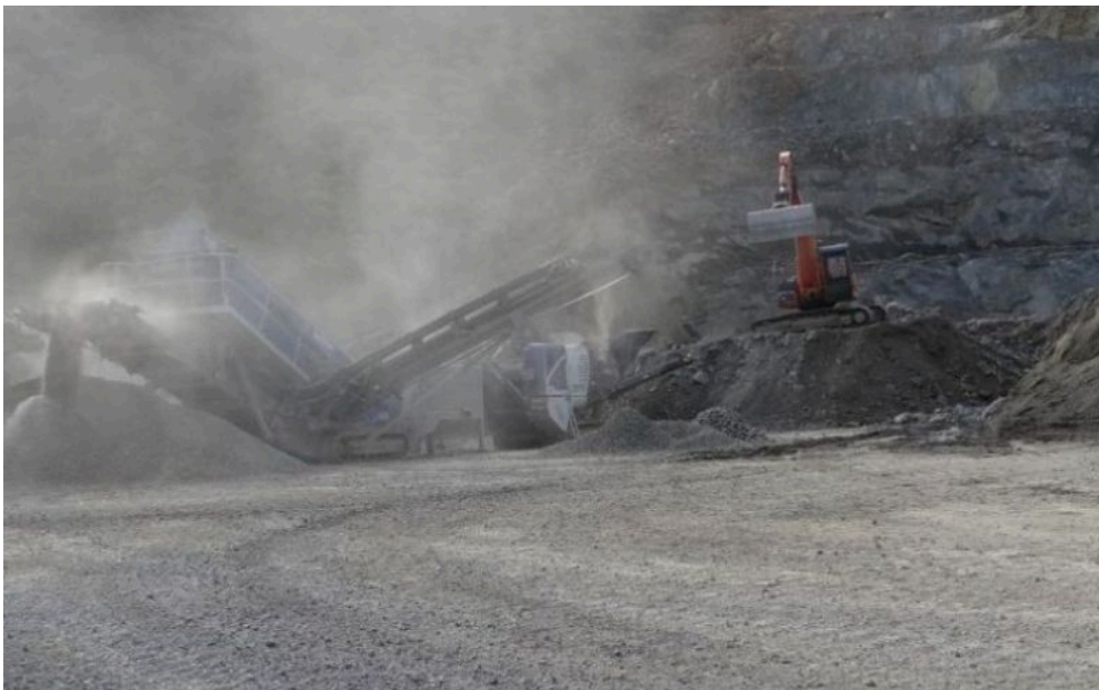
Not that unusual of a sight – unsuppressed dust in a quarry operation.
