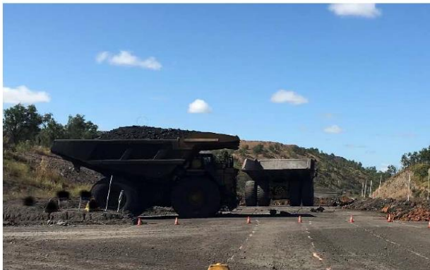
The headboard on the loaded truck would fit beneath the headboard of the empty truck.
