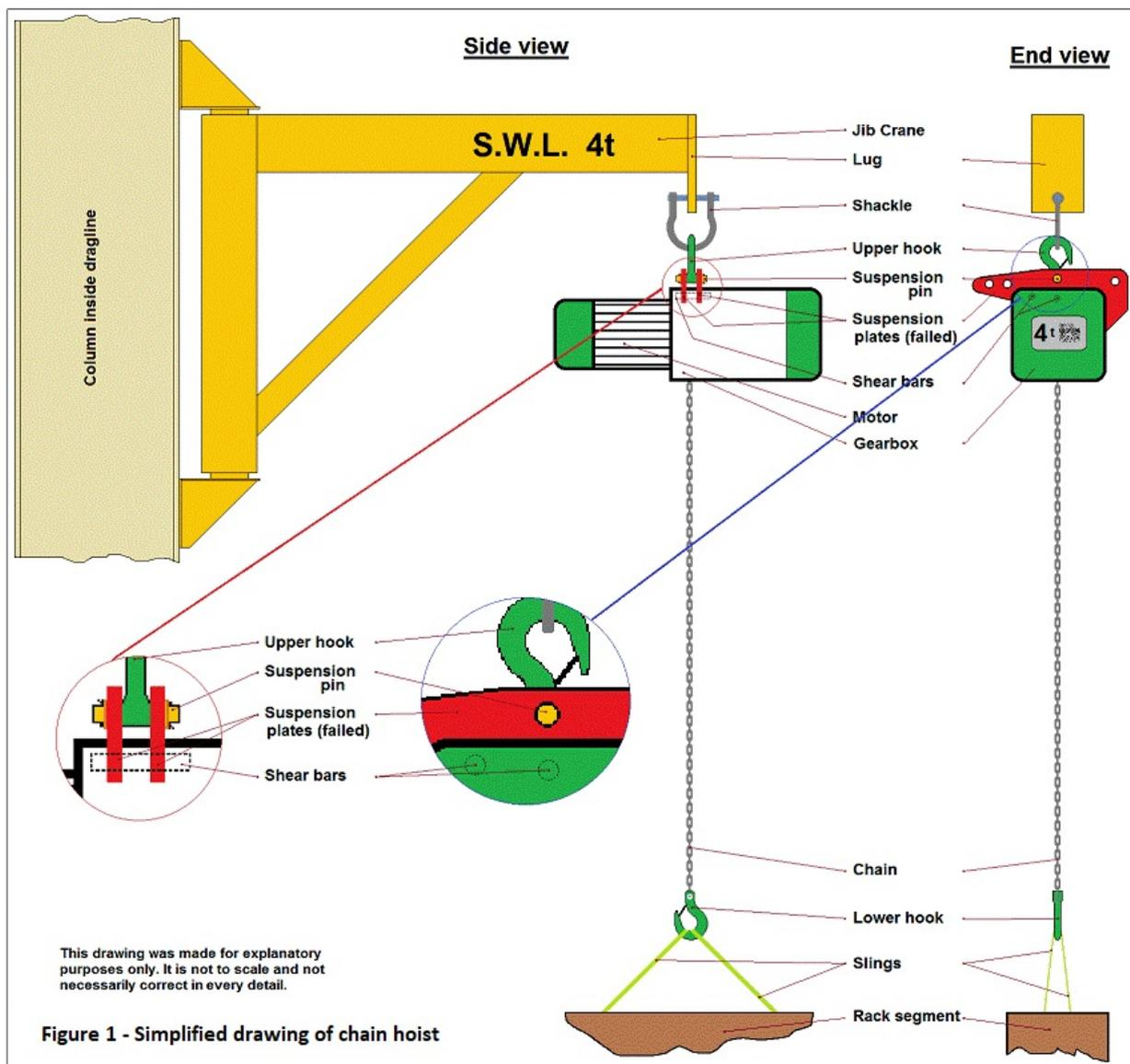
Closer examination revealed that the suspension pin holding the hook had pulled through the sides of the suspension plates. (See Figure 2)
