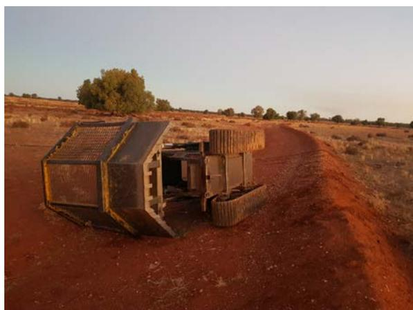
When attachments are designed, an assessment of the effects on the stability of the machine must be completed. This should be reviewed by the mine while undergoing introduction-to-site checks.
