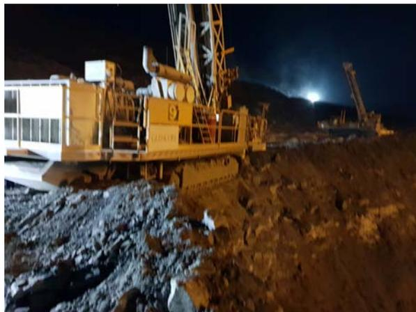
Mine operators should review the management and supervision of trainee drill operators to rigorously manage their exposure to high-risk activities, including drilling the face row near a high wall edge and operating at night or in poor visibility.
