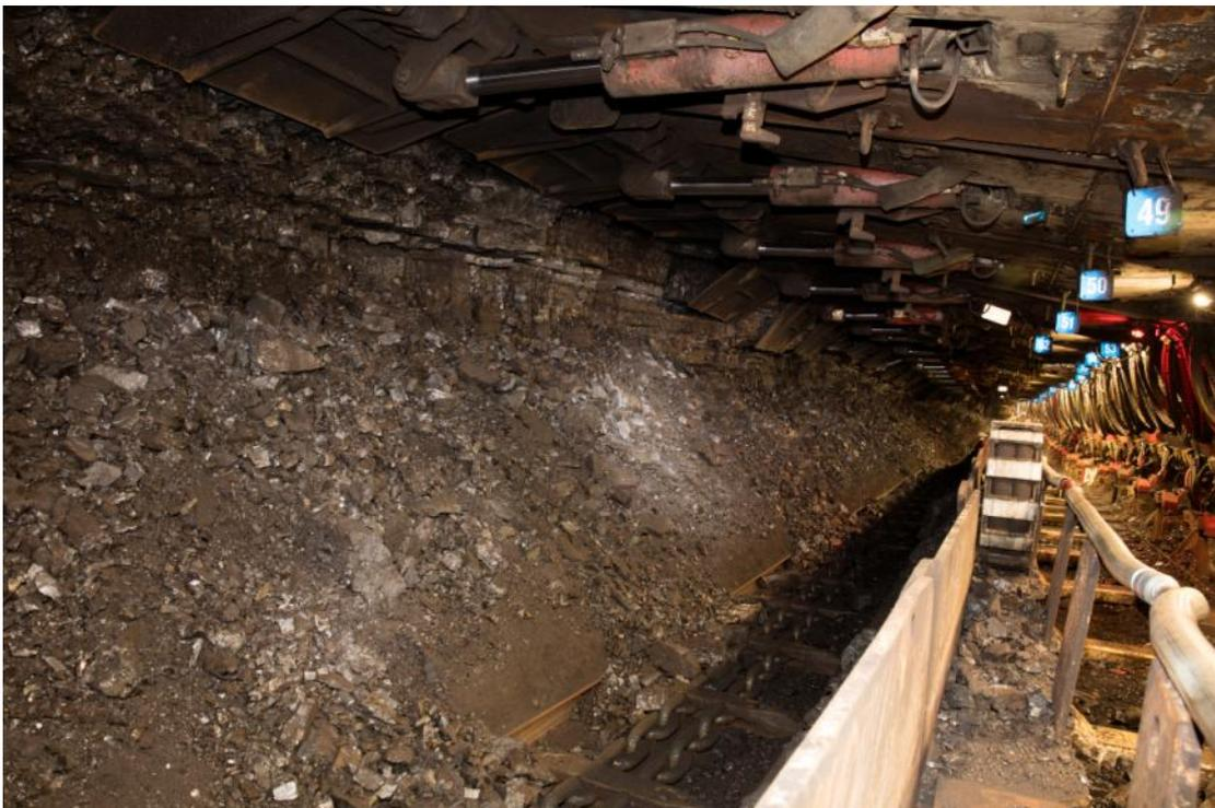
Figure 3: Ejected coal around and between the pontoons of #50 support.
