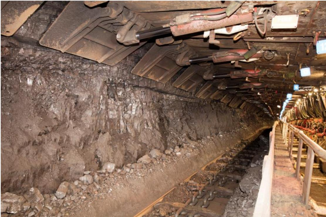
Figure 2: Face condition in burst area, showing the depth of rib blow out (note that the coal had already been run off the AFC).
